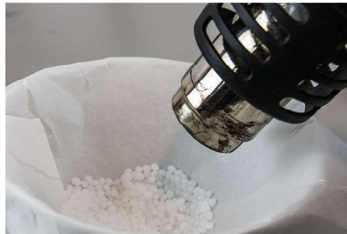
Heat evenly with a heat gun (you can also use hot water)
