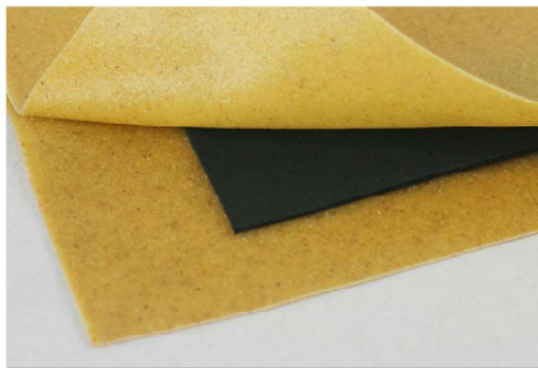
Sandwich EVA foam between hot Worbla sheets
